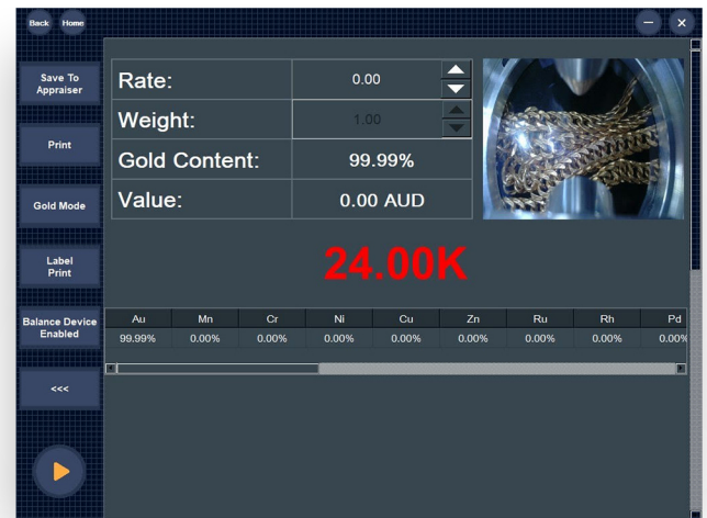
The N1 analyzer displays karat results
